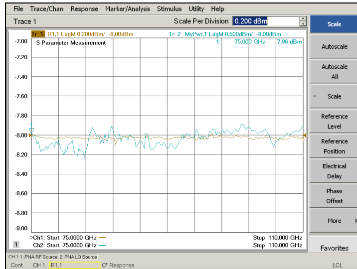
Figure 1. A demonstration of power accuracy; power sensor measurement vs. N5247A PNA-X R1 receiver < 0.1 dBm
